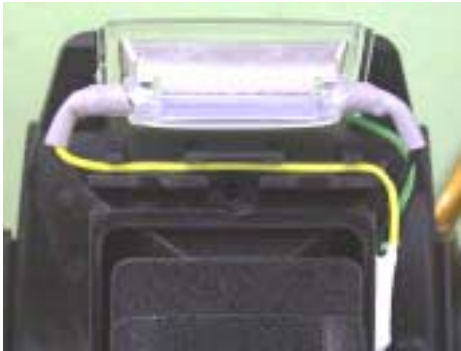
Fig. 8 Arrange lead wires
